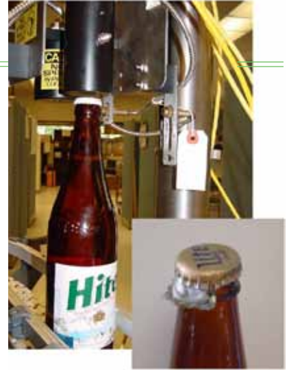
▲ A beer bottle passes under the inspection station of the T500-AC. The inset shows a crown defect.
