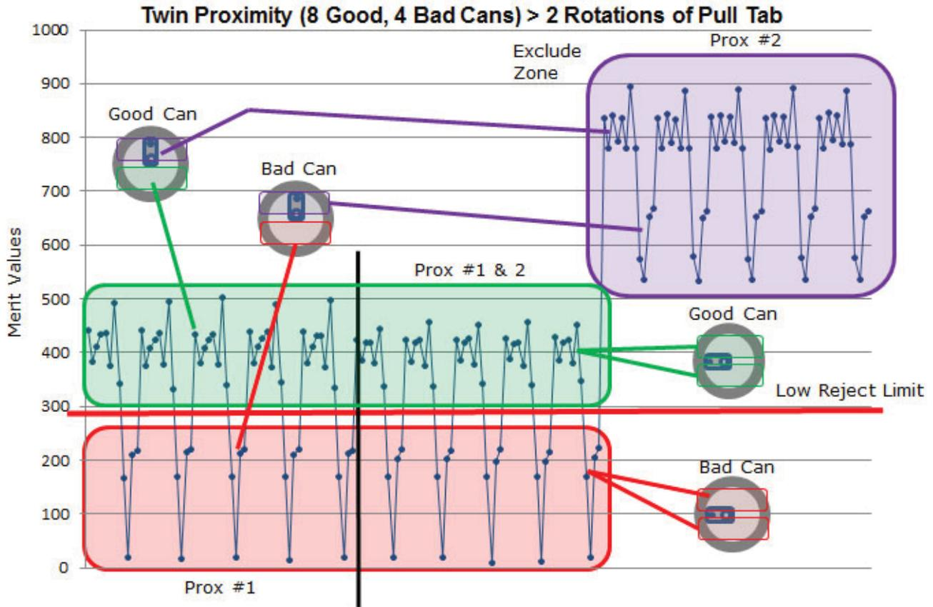
**SUMMARY** Through the use of this innovative proximity sensor system, the TapTone twin proximity sensor eliminates the negative effects of random pull tab orientations on mixed metal EZ open can ends (steel vacuum cans with aluminum pull tabs). This sensor is only available for use with the new Teledyne TapTone T550 and PRO Series user interfaces. Contact your local TapTone Agent for more details on this new and exciting technology for vacuum can inspection.
