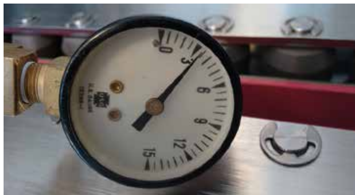
▲ Gauge showing the low internal pressure during inspection.
