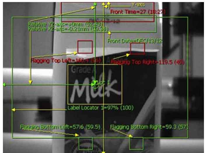
Missing Digits in Front Time Stamp and Flagging Label Detection
