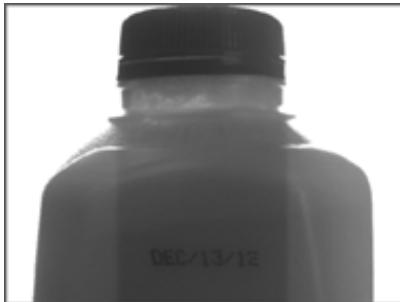
▲ Fig. 2b Camera 2 –Rear cap and date code of a one quart milk container
