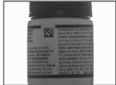
▲ Fig. 3c Camera 3 –Back 2D barcode/2D data Matrix of a 60 tablets container of Cetirizine HCl/Antihistamine
