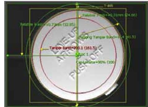
Missing Tamper Band Detection
