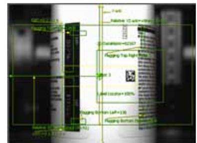
▲ Fig. 4d Camera 4 –Date and lot code, and 2D barcode / 2D data matrix of a 100 caplets container of Acetaminophen
