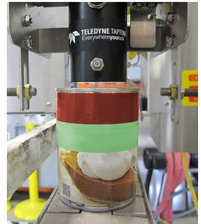
A can of evaporated milk passes under the RTV-P sensor
