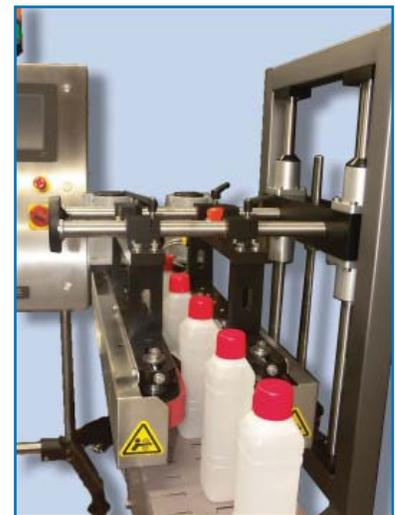
T-4000 Compression Controller and Sensor. Sensor has a cantilever design that suspends over the existing conveyor.
